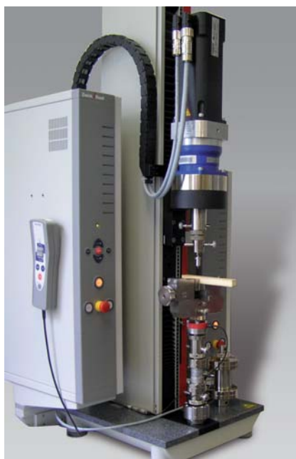
Fig. 3: zwicki-Line with torsion drive
