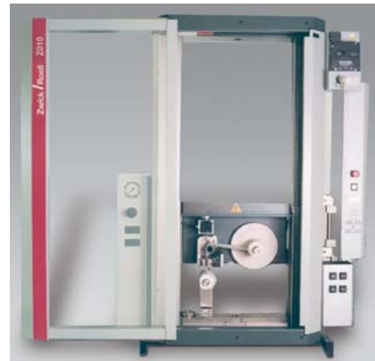
Fig. 3: Unrolling test for gauze bandages
