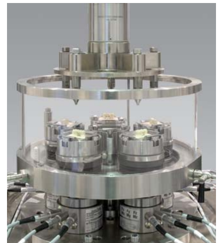
Fig. 4: Test kit for dental implants (Dental Clinic, University of Ulm)
