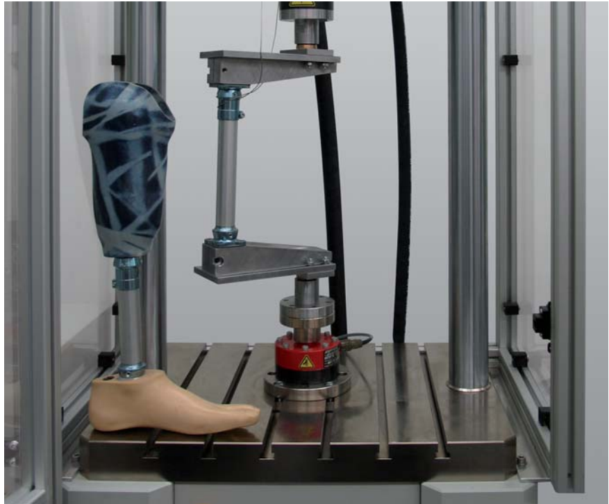
Fig. 1: Test device for lower-leg prostheses
