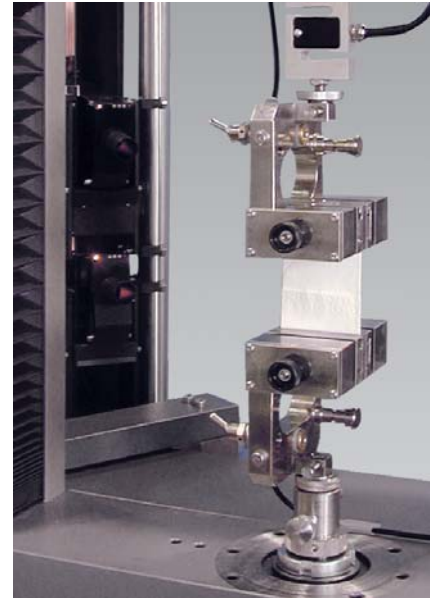
Fig. 5: Tensile test on non-wovens
