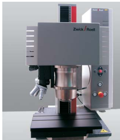
Fig. 2: Fully automatic Zwick/ZHU2.5/Z2.5 universal hardness testing machine with motorized displacement unit
