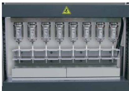
Fig. 3: Device for simultaneous testing of up to 8 hypodermics
