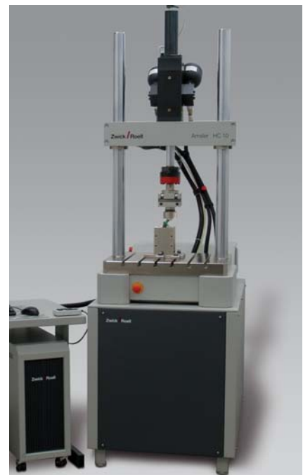
Fig 2: Servo-hydraulic testing machine Amsler HC-compact
