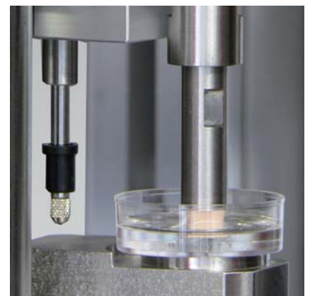
Fig. 3: Compression test on bone replacement material
