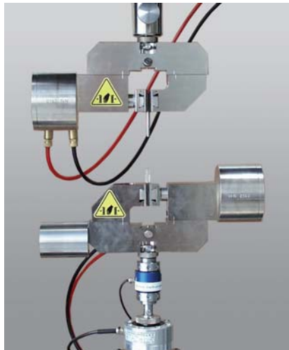
Fig. 2: Testing luer-lock connections
