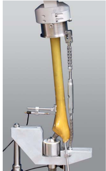
Fig. 2: Specimen grips for tests on endoprostheses
