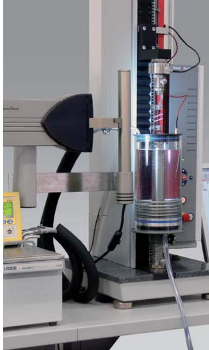
Fig. 1: zwicki-Line with temperature-controlled fluid bath and videoXtens (bath lowered for specimen change)
