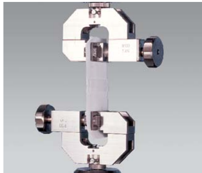
Fig. 3: Testing seam slippage resistance
