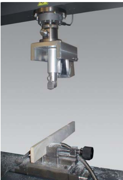
Fig. 1: Device for compression tests on sagittal saw blades
