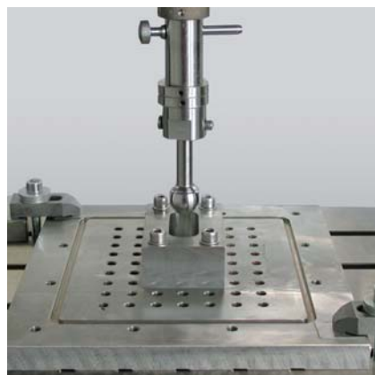
Fig. 2: Torsion test on artificial hip-joints
