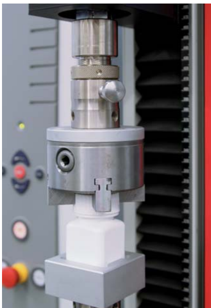
Fig. 1: zwicki-Line Torsion for push & turn tests on pharmaceutical packaging
