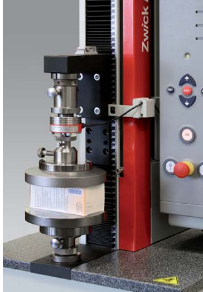
Fig. 2: Compression test on cardboard packaging
