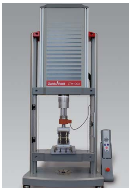
Fig. 1: LTM1000 with spinal implant
