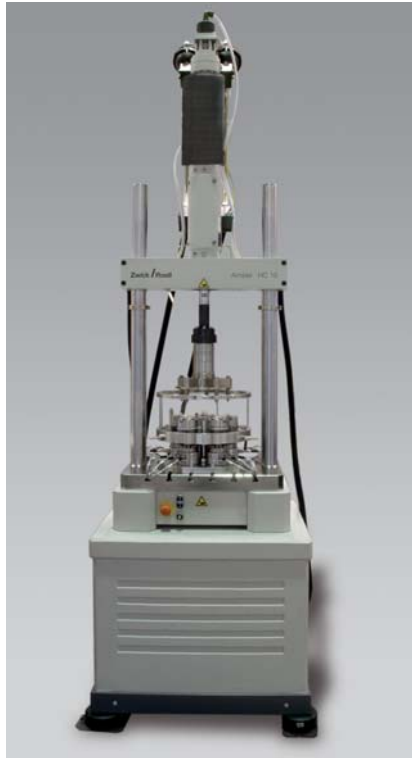
Fig 1: Servo-hydraulic testing machine Amsler HCT 10/100
