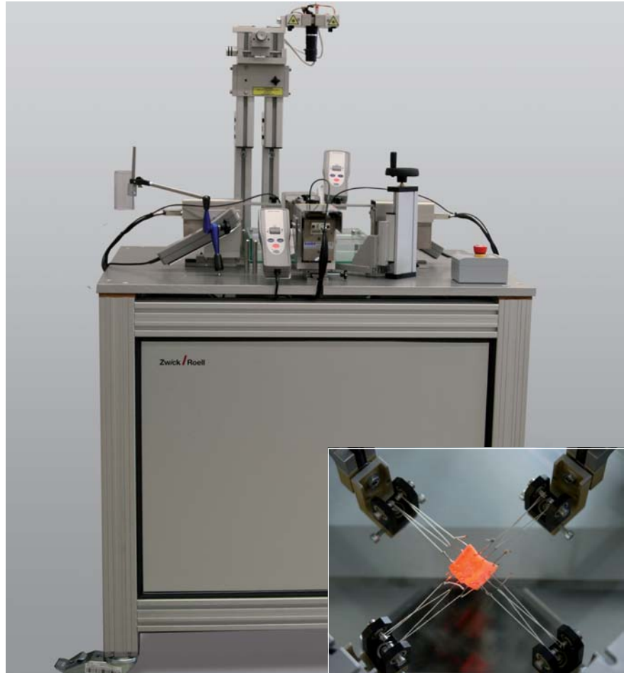
Fig. 1: mediX0.1 biaxial materials testing machine with integrated laserXtens. Inset.: Specimen grips for biaxial tests on biomaterials
