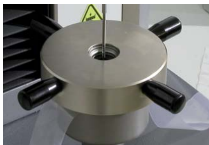
Fig. 1: Foil retainer for penetration force measurement
