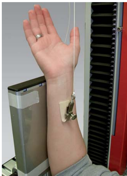
Fig. 1: Peel test on wound dressings
