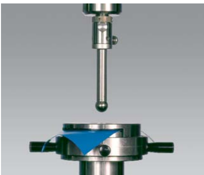
Fig. 2: Testing burst strength
