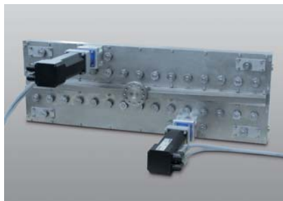
Fig. 2: Test device for stents
