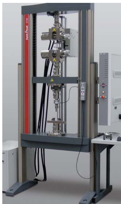
Fig 1: Allround-Line floor-standing machine Z100
