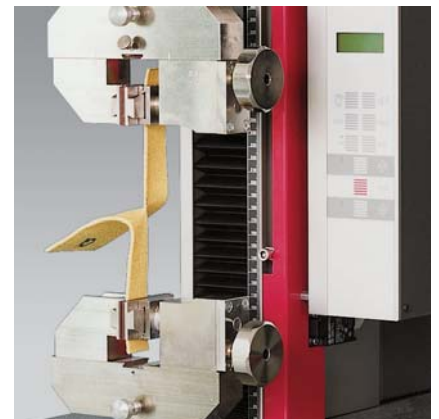
Fig. 4: Tear growth test on plastic film
