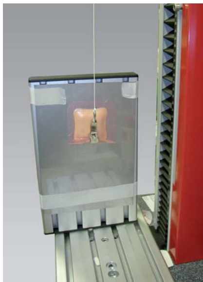
Fig. 2: Determining adhesive forces of wound dressings
