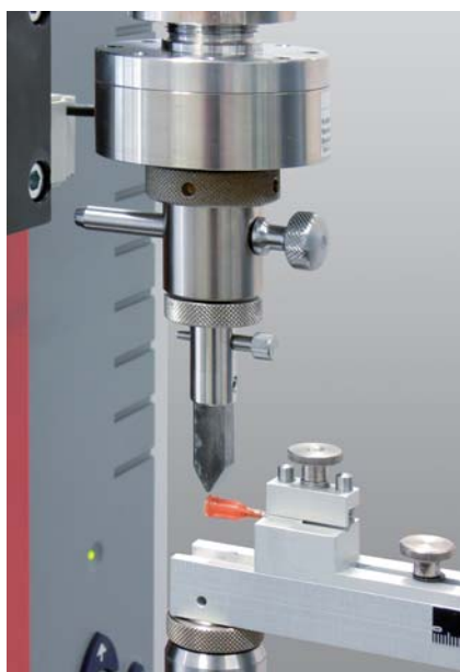
Fig. 1: 2-point flexure test kit for testing hypodermic needles
