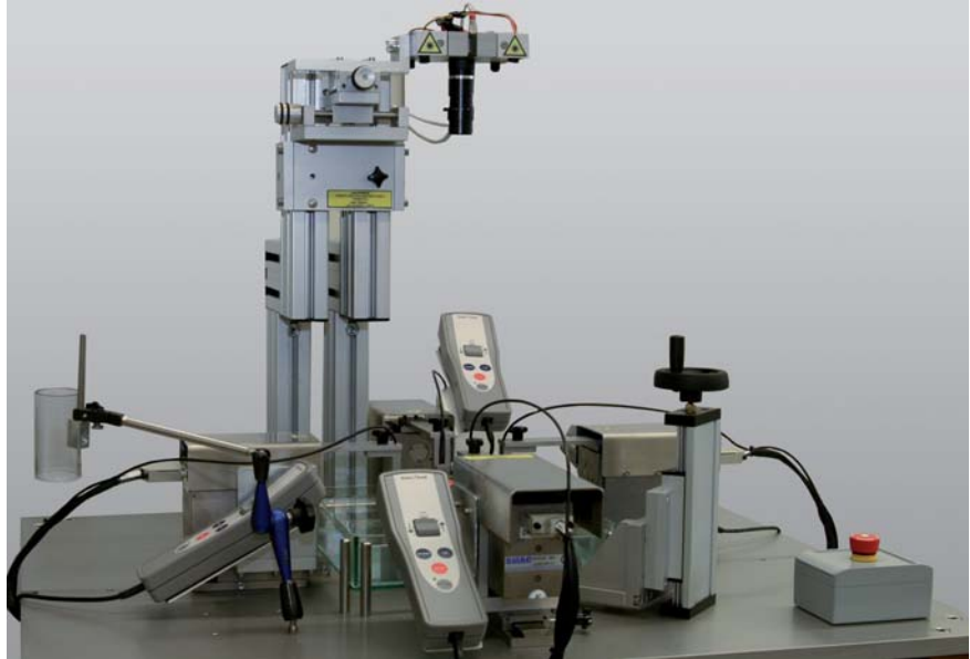
Fig. 1: mediX0.1 biaxial materials testing machine with laserXtens
