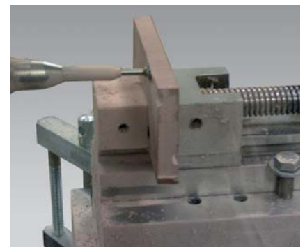
Fig. 2: Penetration test on bone drill
