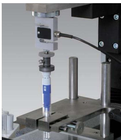
Fig. 1: Discharging device for testing insulin pens
