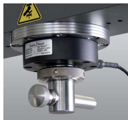
Fig 2: Load cell Xforce; design: multiple strain-gage
