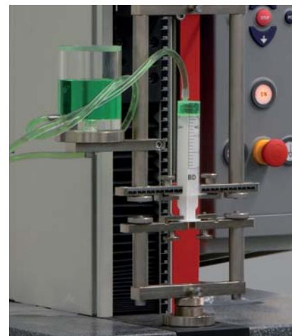
Fig. 4: Determining hypodermic plunger actuation force
