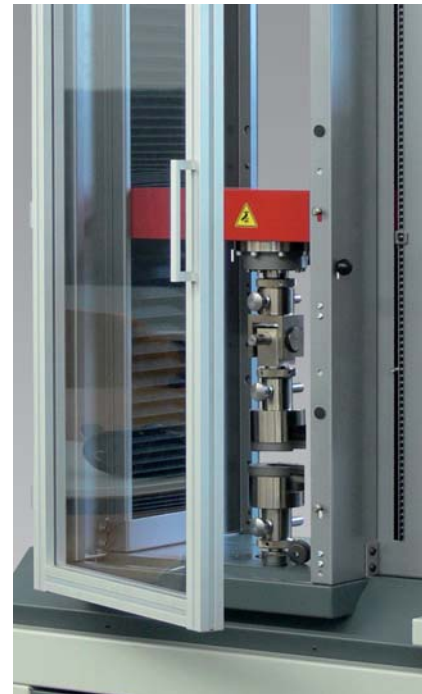
Fig 2: ProLine Z050TN with CE conforming protective screen
