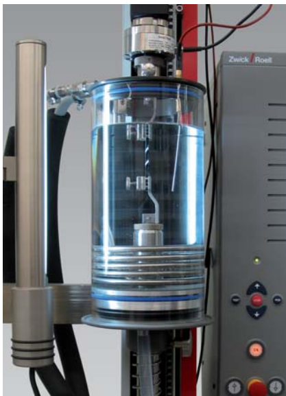
Fig. 1: Media container with temperature control unit
