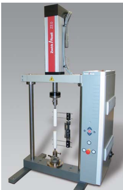
Fig. 2: Electromechanical servo testing actuator with external fixation of fractures
