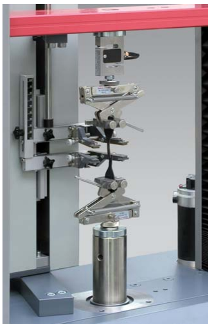
Fig. 1: Tensile test on rubber raw material
