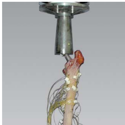
Fig. 2: Femur with implanted endoprosthesis and with strain gages applied
