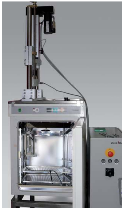
Fig. 2: Integration of a temperature chamber into the test arrangement
