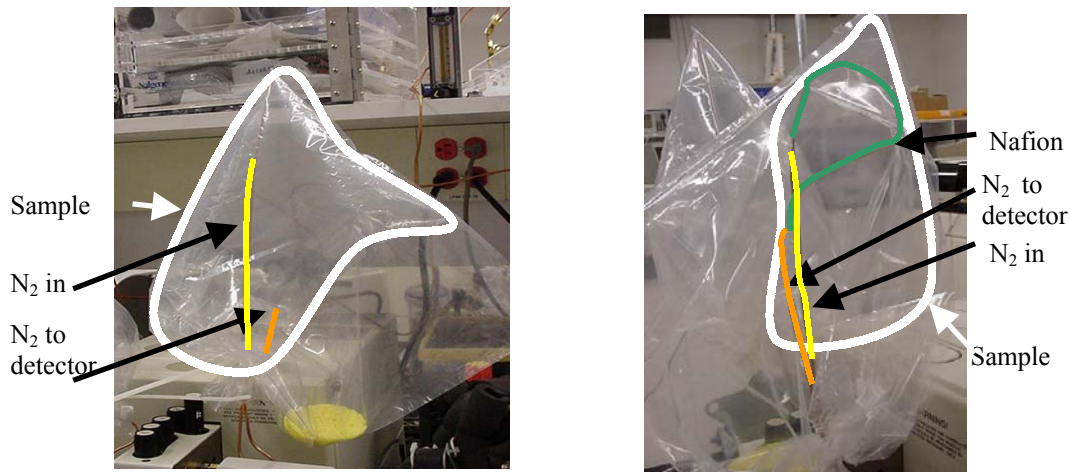
Figure 4. Experimental set-up used to compare water vapor transmission rate results with and without nafion tubing.
