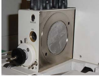
Figure 2. Screen placed in dry chamber of diffusion cell
