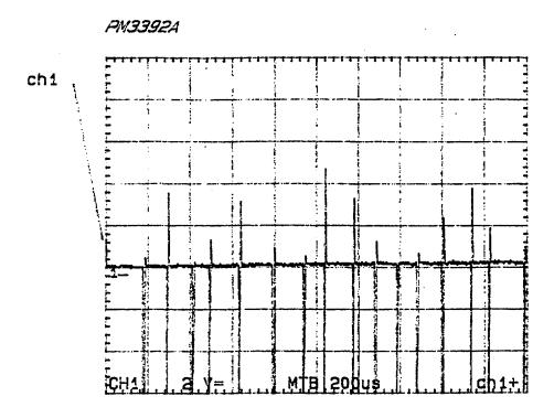
FIGURE 3. AMPLIFIER OUTPUT IN TEST 1
