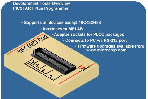
Once you have code up and running through either the emulator, the debugger or simulator, you will need to program your devices. The PICSTART Plus is a very convenient universal desktop development programmer that supports all devices except the 16C432/433 devices, and also runs under the MPLAB IDE.
