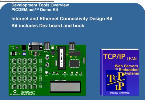
The PICDEM.net<sup>™</sup> is an Internet and Ethernet demonstration kit that is designed to show internet connectivity capability using PIC MCUs. The complete kit includes a demonstration board with TCP/IP stack and a book written by Jeremy Bentham which explains the basics of small TCP/IP Internet connectivity and web servers, along with the basics on how to implement those on a 8-bit embedded systems.
