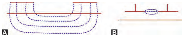
Figs 4.14A and B: Coplanar arrangement of electrodes: (A) Correct spacing and (B) incorrect spacing
