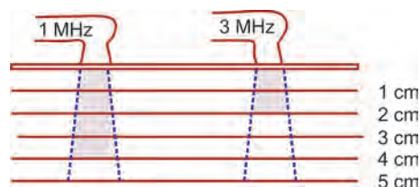
Fig. 8.3: Depth of penetration of ultrasound waves
