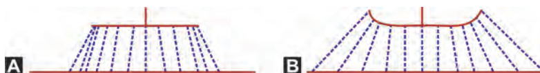
Figs 4.4A and B: Electric fields produced by Flat (A) and (B) Convex electrodes
