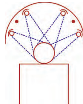
Fig. 5.5: Theraktin tunnel arrangement of fluorescent tubes
