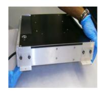
Step 3 – Lightly, re-install the fasteners and secured them as required.
