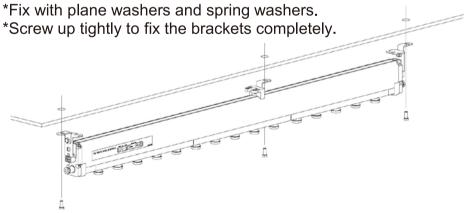
② Set up angle, screw up M5 screws tightly.
