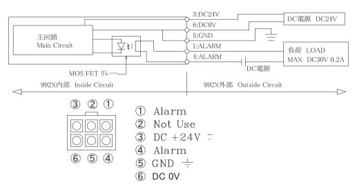
\*Securely connect the ground wire to the ground. (type a or type b). \*Use the LPS(Limited Power Source) certified with IEC/EN60950-1.
