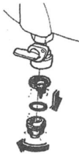
Fuel Filter Element Removal
