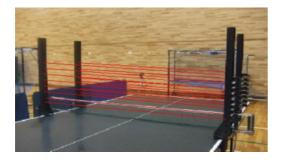
Feg.1 The system of the two infrared sensors was fixed 0.3 m from the net respectively.
