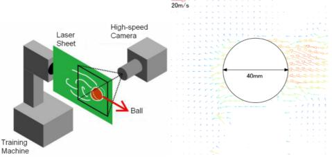
Fig.1 Schematic view of Experimental Setup
