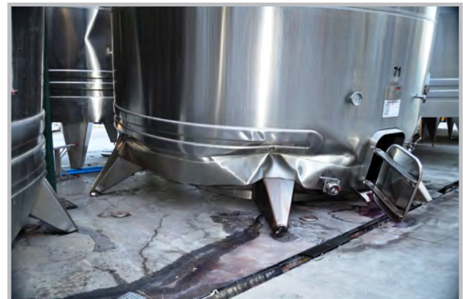
Close-up of the support failure in a cylindrical stainless steel wine storage tank (Source: RMS)
