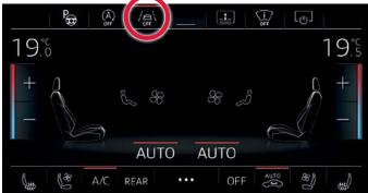
Positioning of the virtual button for activating and deactivating the lane departure warning
