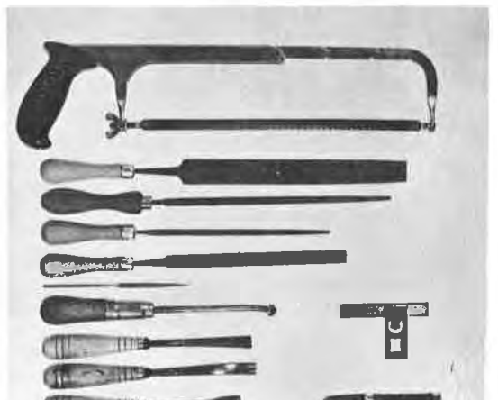
17 Assortment of tools used for conversion shown. Files and rasps are for shaping stock and metal work. Small Swiss files, offered singly and in sets, are particularly useful for final shaping of trigger guard, etc., and for finishing sharply curved-surfaces around pistol grip, cheek-piece and comb. Scraper with round cutter head is handy tool for precise inletting of barrel into forearm
