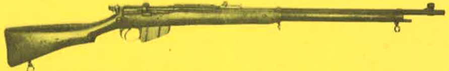
3 Charger-loading Lee-Enfield Mk. I* (CLLE), or long Lee-Enfield. Weight about 9.4 lbs., over-all length 49½", barrel length 30¼". This model, an improvement of the magazine Lee-Enfield Mk. I (MLE) introduced in 1895, has safety lock which appeared in Lee-Enfield Mk. II* in that year, and deep broad-land rifling required to resist cordite erosion. Charger-loading guides were added to existing rifles in 1907
