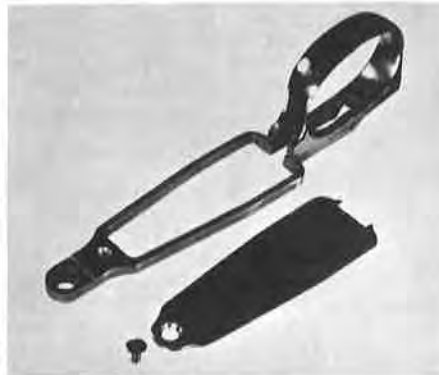
11 Appearance of trigger guard is enhanced if guard loop is modified by filing as shown. Floorplate made from sheet metal is retained by single screw and notch filed in guard loop. Top of floorplate can be filed to arched contour of factory-made plate. Forepart of guard tang shown was rebated to eliminate unsightly punch marks around guard screw hole
