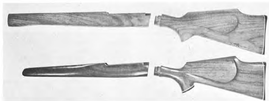
4 Typical semi-inletted (upper) and finished (lower) SMLE stocks as furnished by E. C. Bishop & Sons, Inc., and other U. S. stock firms. Only minor inletting is required to fit finished stock to rifle. Most stock suppliers will fit semi-inletted stock to customer's barreled action at nominal cost
