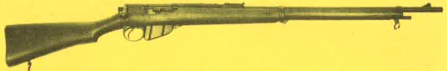
2 Lee-Enfield Mk. II. Weight about 9 lbs., over-all length 49½", barrel length 30¼". Rounded-corner rifling of Metford type originally devised to minimize black-powder fouling, and appropriate in this rifle since original .303 loading was compressed pellet of blackpowder. This model, introduced in 1892, differs from original Mk. I of 1888 principally in 10-round instead of 8-round magazine and in simplified bolt. Smooth outline of action top is due to absence of charger-loading guides and to steel dust cover which moves with bolt
