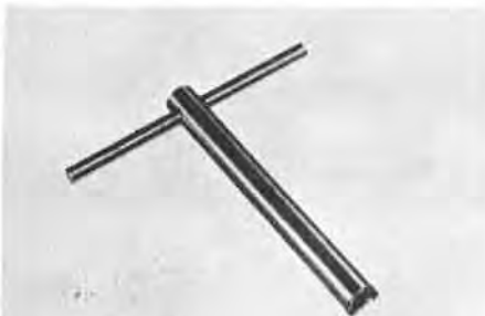
16 Spanner wrench made from short section of \frac{3}{8} " steel rod is required for bolt disassembly and assembly. Drill \frac{3}{16} " hole in center to depth of 1\frac{1}{4} " and file twin lugs on end to engage notches on side of firing pin. Wrench is used through front of bolt after unscrewing bolt head and removing locking screw from rear of cocking piece
