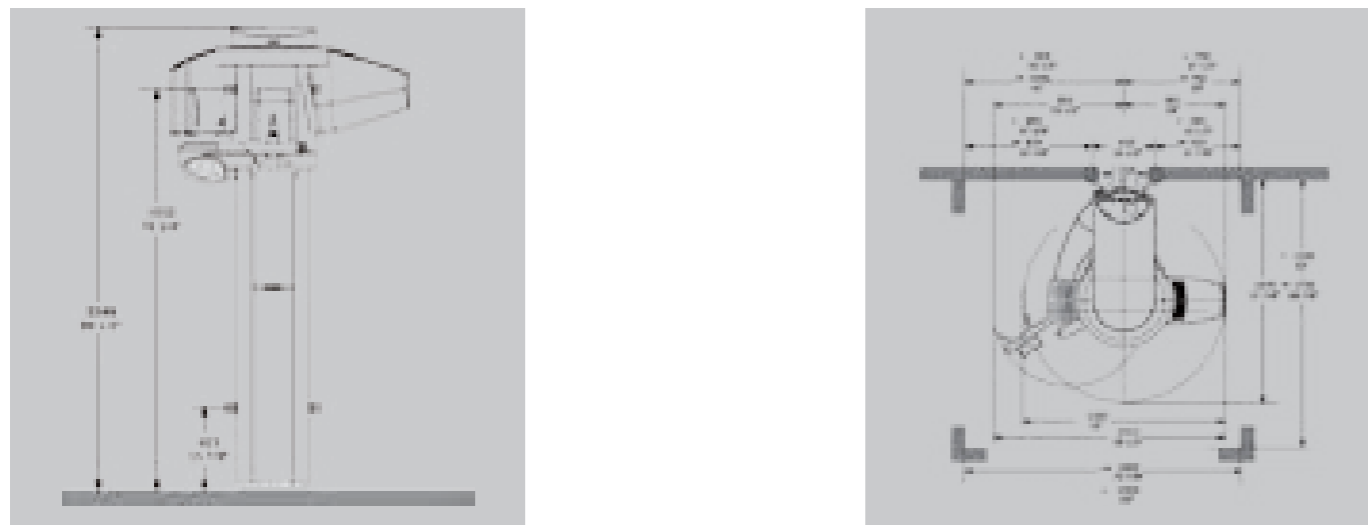
Galileos Comfort Plus: Space requirement at least 1,600 mm x 2,250 mm
