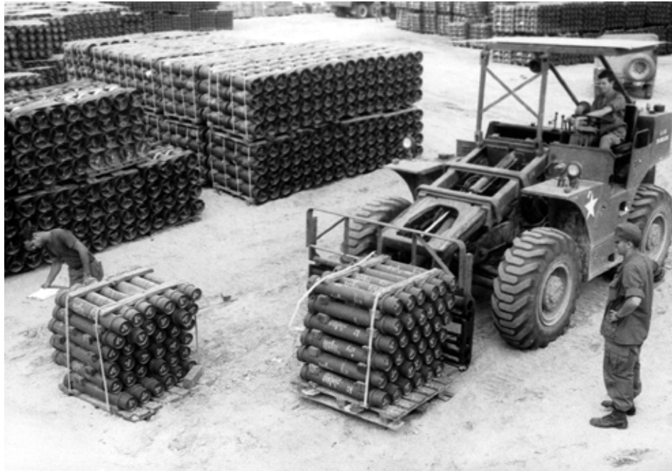
The 6,000 pound rough terrain forklift was a vital part of ammunition supply operations. Each ASP relied on the heavy duty machines for loading, offloading, and internal movement of ammunition and heavy ordnance. At Chu Lai ASP, 295th Ordnance Company Private First Class Dennis Schuyler (far left) checked lot numbers before Sergeant Warren Hinzie moved the pallets in January 1969.
