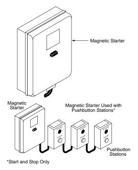
How the Non-reversing Magnetic Starter Works
