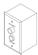
This is just like the light switch. It only turns the conveyor ON and OFF.
