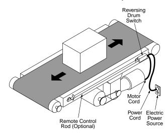
Disadvantages of a Manual Reversing Drum Switch
