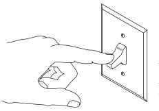
It controls the lights in each room. It turns the electric power to the lights ON and OFF.
