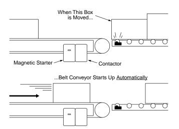
A contactor is another type of electrical control used with Limit Switches and Magnetic Starters.
