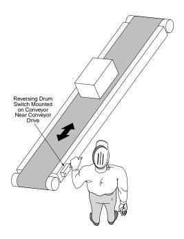
2. With remote control rod...conveyor can be controlled from EITHER end.
