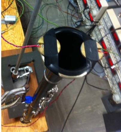
Figure 6: The apparatus for the longitudinal mechanical resonance experiment involved clamping the clarinet upside-down by the thumb rest to a ring stand using electrical tape and a C-clamp. Two piezoelectric transducer discs were placed on the bell of the instrument to induce and measure mechanical vibrations.
