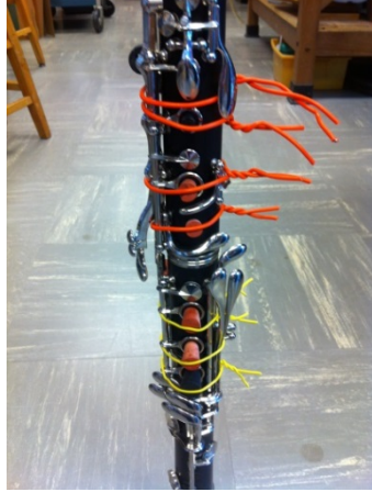
Figure 4: Rubber stoppers and PVC-coated wire was used to close the tone holes necessary for specific notes tested. This picture shows the wooden Buffet R-13 Bb clarinet configured for concert F_3 before doing a frequency spectrum impedance analysis.
