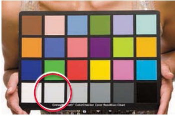
Figure 4.22 The X-Rite ColorChecker Classic chart. To take a white balance reading in Lightroom, click the light gray patch next to the white patch.
