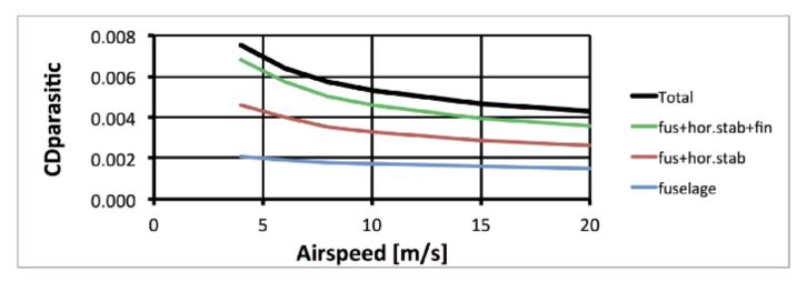
Figure 9: Build-up of the Parasitic drag.
