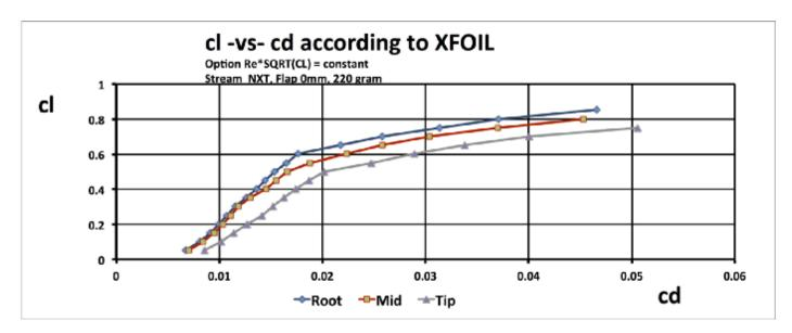
Figure 7. Example calculated airfoil properties for flap deflection of 0 mm
