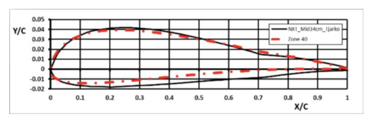
Figure 13: Comparison geometry measured NXT airfoil at 34 cm from the root with the V1 Zone — 40 airfoil.
