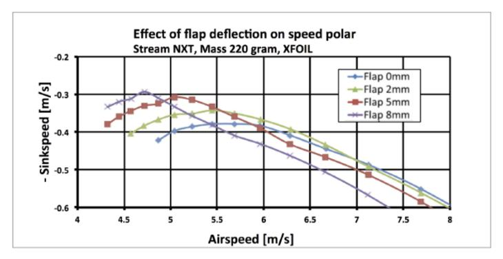
Figure 10: Effect of flap deflection on the speed polar.
