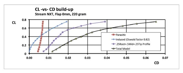
Figure 8: The main drag coefficients, non-dimensionalised with dynamic pressure and wing area.
