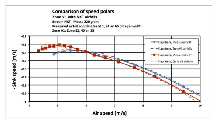
Figure 14: Comparison of speed polars.
