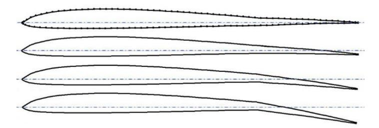
Figure 6: The geometry of the airfoil at 34 cm wingspan with flaps 0, 2, 5 and 8 mm
