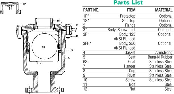
\*Part No's 1P, 1S, 3, 3F and 3H are at customer's option. \*\*For ease of maintenance, some of the above parts are provided as kits or assemblies. \*\*\*Note: Prices and Materials are Subject to Change Without Notice
