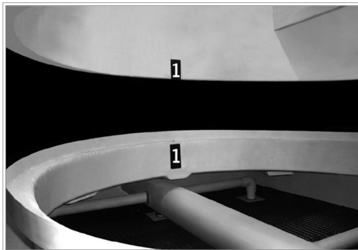
Figure A-37: Fan adaptor alignment
