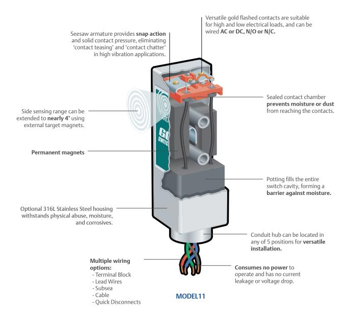
Models 11, 21, 31, and 81 were the world's original GO Switches. Their simple design, rugged housings, long sensing ranges, and global approvals make these switches the ideal choice wherever reliable proximity sensing is needed. Some features common to all these models include a standard operating temperature range of -50 °C to 105 °C (-58 °F to +221 °F) and gold-plated SPDT dry contacts.
