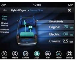
Hybrid screens. Uconnect offers Hybrid Electric Pages on the Driver Information Display (DID), providing customizable efficiency and power-usage details.
