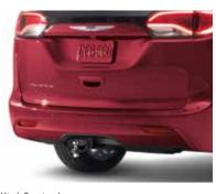
Hitch Receiver.\* Receiver increases towing capacity to up to 1,800  $\ensuremath{\mathsf{lb}}$  with weight-distributing equipment. The Hitch Ball, Ball Mount and Wiring Harness are sold separately.
