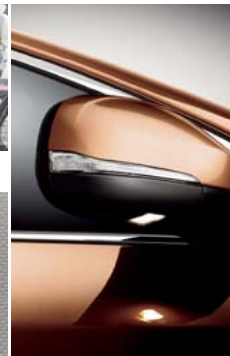
Power retractable door mirrors with ground lighting (Retractable function only with BLIS option)
