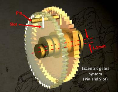
The movement of the Moon is not circular but elliptical. The Mechanism's display of this movement takes into account the anomaly caused by its eccentric orbit around the Earth by using two eccentric gears, the axes of which are separated by 1.1 mm. The lower gear has a pin that engages with a slot on the upper gear, forcing it to rotate elliptically. The epicyclical movement of the upper gear tracked the motion of the Moon in the sky with great accuracy.
