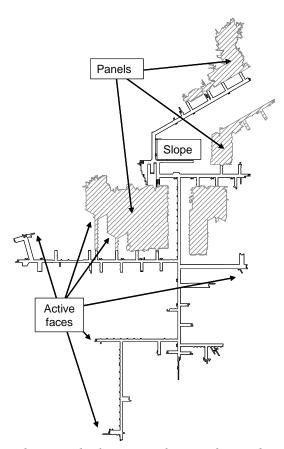
Figure 25 - Mine Ga layout showing the location of active faces, the slope and panels within one active level.
