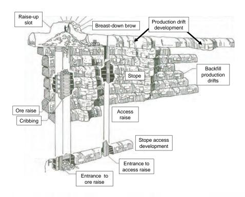
Figure 36 - Diagram of Captive Cut-and-Fill mining method.
