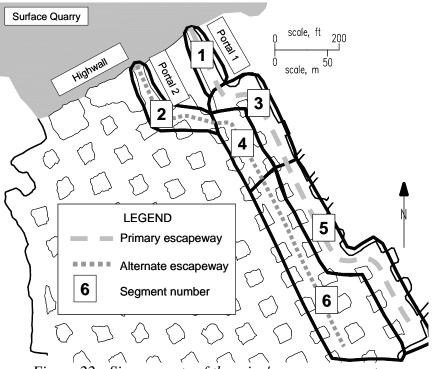
Figure 22 - Six segments of the mine's escapeway system.
