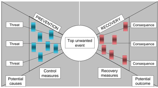
Figure 8 - Bow Tie Analysis (BTA) method.
