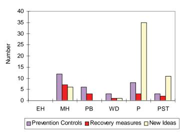
Figure 38 - Distribution of prevention controls and recovery measures for the captive cut-and-fill change of mining method risk assessment.
