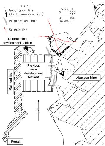
Figure 19 - Techniques used to find the location of water-filled old mine workings at Mine Ea.
