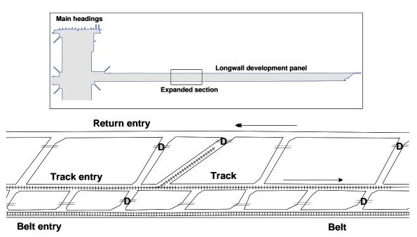
Figure 34 - Site conditions at Mine I showing the 3-entry development panel with direction of air flow.
