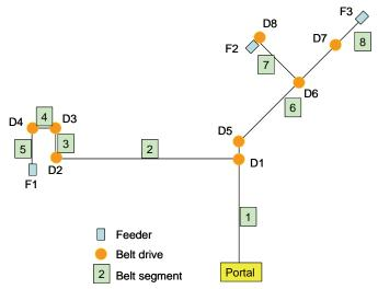
Figure 31 - Segments of the conveyor belt system.
