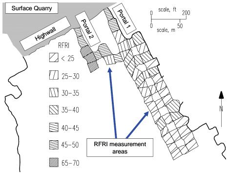
Figure 23 - Roof Fall Risk Index (RFRI) measured in the mine's escapeways.
