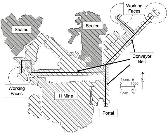
Figure 30 - Mine H layout showing the location of the conveyor belt and working faces.
