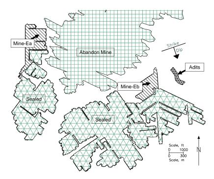
Figure 16 - Location of Mines Ea and Eb and adjacent water-filled abandoned mine and water/gas filled adits.
