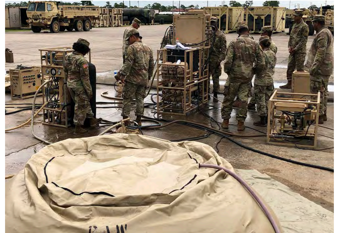
Quartermaster and Chemical Equipment repairers and Tactical Power Generation specialists conduct technical inspections on Lightweight Water Purification Systems to build equipment readiness at Fort Stewart, Georgia, on Oct. 6, 2022. (Photo by Chief Warrant Officer 2 Rickey Ivey)
