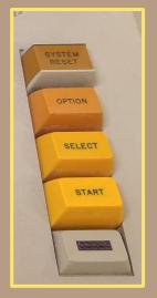
**System Reset:** This key will stop any programs currently running and reset the computer.
