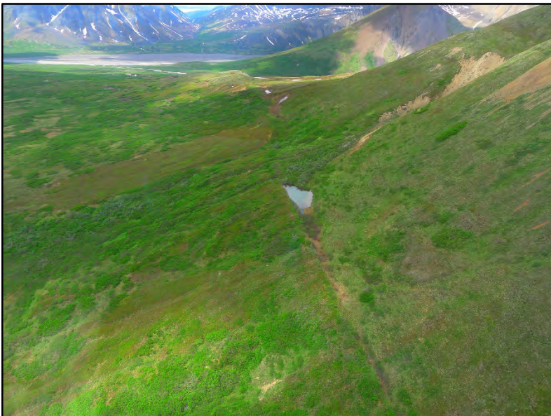
The Denali fault extends through the pond in the center of the photo and is marked by a distinct break in the surface. Paleoseismic studies indicate that this part of the fault generates large earthquakes every 250-400 years; however, the locations of microseismic events along the fault, particularly west of Denali National Park, are poorly constrained due to limited seismic monitoring stations.
