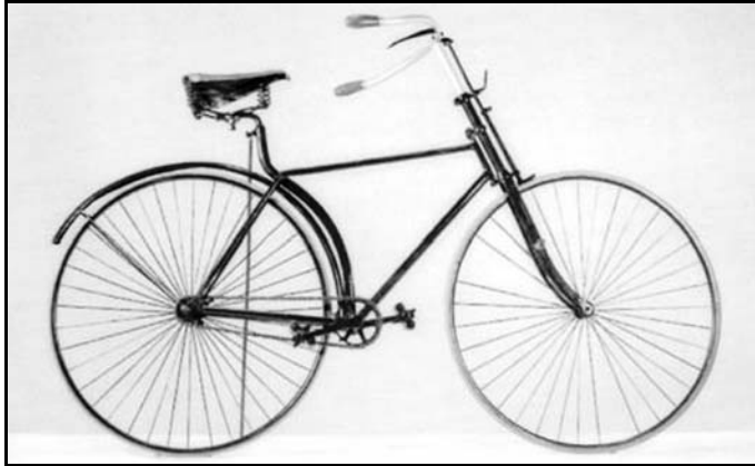
A “safety” bicycle from around 1886/7, with hard tyres.
