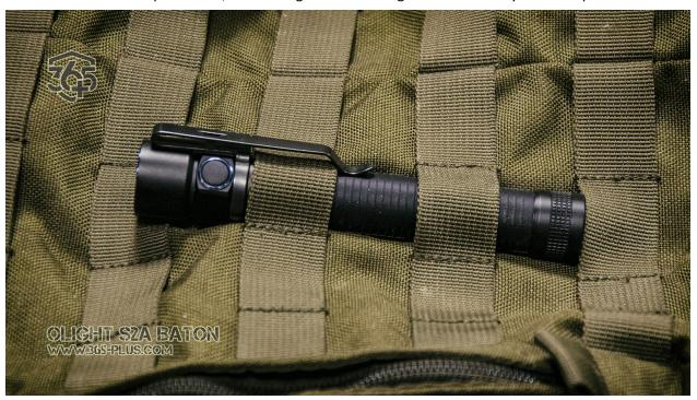
The button is a multi-functional switch. The whole operating of the flashlight is done through a single button. Powering ON/OFF and mode selection can all be done without changing the grip. Single click for power ON, hold button when ON to cycle through power modes and single click for OFF. When OFF, hold button for 1 second to access 0,5 lumen "moonlight" mode. The flashlight stores the last setting and uses it when you power it on the next time.
