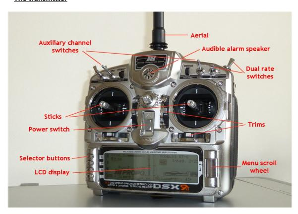
The transmitter is the heart of the radio control system and is the box that you hold and use
