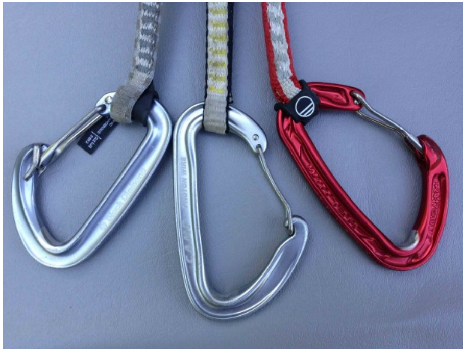
Three different options for keeping the lower carabiner in its proper orientation, left to right: Sewn-in rubber positioner on the Black Diamond Oz, sling sewed tight around the bottom for the Camp Photon Wire Express, and an exterior positioner on the Wild Country Helium.
