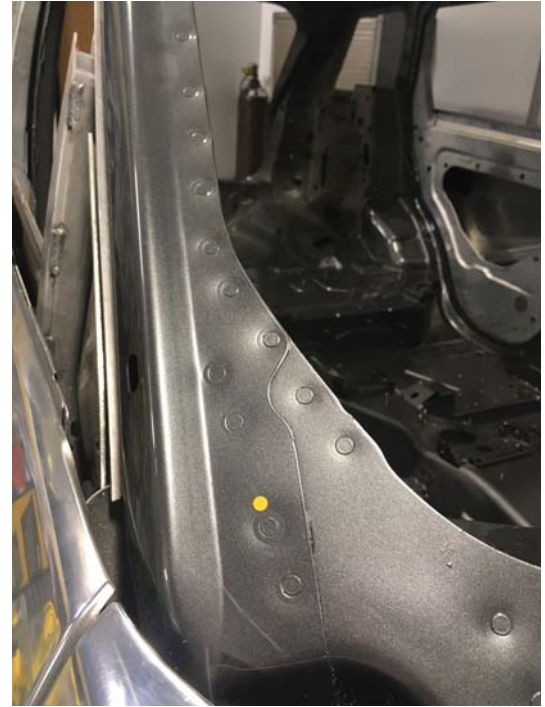
STANLEY Engineered Fastening self-pierce rivets used to join pieces of Range Rover B-pillar.
