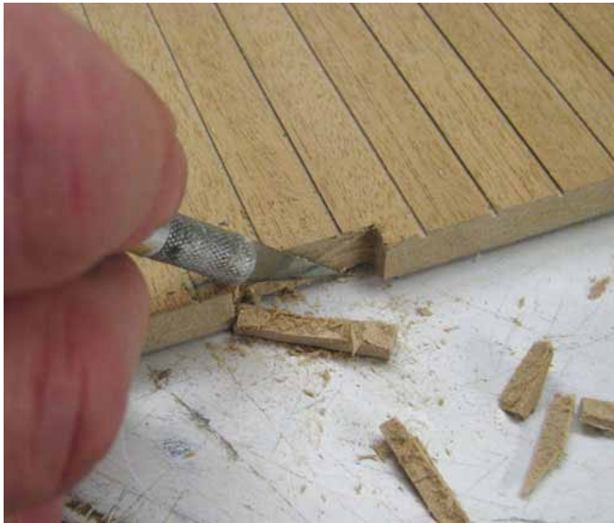
Cutting an Electrification Slot before building
