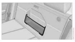
A storage compartment is located behind the rear seat backrest. To access the storage compartment: remove the insert or fold down the rear seat backrest.
