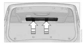
The warning triangle is located in a holder in the trunk lid. Press the tabs to take it out.
