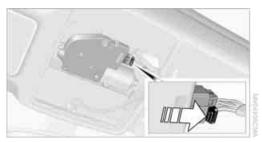
Insert the Allen wrench supplied with the onboard vehicle tool kit, refer to page 270, into the opening provided. Move the glass roof in the desired direction.
