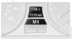
The selector lever position and the engaged gear are displayed, e.g. M4.
