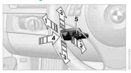
Press the lever upward or downward, arrow **3**. The displays on the speedometer disappear. In addition, the system is automatically deactivated:
