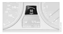
The car's current speed is stored. It is displayed on the speedometer and briefly in the instrument cluster.
