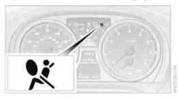
As of radio readiness, refer to page 61, the warning lamp lights up briefly to indicate that the entire airbag system and the belt tensioners are operational.
