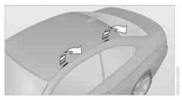
The mounting points are located in the roof.
