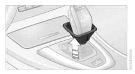
Using the allen wrench from the tool kit, refer to page 270, rotate the cover until it reaches the stop, arrow 1, and remove, arrow 2.
