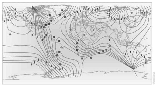
To set the compass zone, press the adjustment button for approx. 3-4 seconds. The number of the compass zone set is shown in the display.
