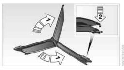
Press together the top and bottom parts of the wind deflector until the catch engages, arrow 2.
