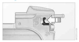
Slide the red release lever towards the middle of the wind deflector and push the two halves apart.
