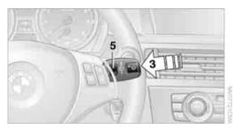
Press the button, arrow **3**. The LED in the button lights up.
