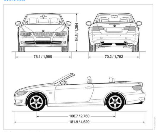
All dimensions given in inches/mm. Smallest turning circle dia.: 36.1 ft/11.0 m 335i: height approx. 54.0 in/1,370 mm
