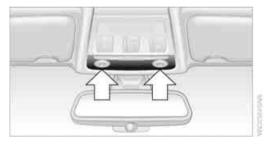
Insert the screwdriver into the openings on each side to press the clips.
