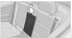
Front cover: press the two recesses together and fold the cover down until it engages.
