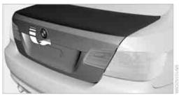
Press the button, see arrow, or the button on the remote control for a longer period. The trunk lid will open slightly. It can now be swung upwards.
