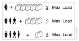
The permissible load is the total of the weight of occupants and cargo/luggage. The greater the weight of the occupants, the less cargo/luggage can be transported.
