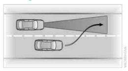
When a vehicle moves from an adjacent lane into your lane, Active Cruise Control will not recognize this vehicle until it is fully in your lane ahead of your vehicle.
