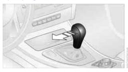
Move selector lever from position D toward the left into the M/S shifting slot; the Sport program is activated. This position is recommended for a performance-oriented driving style.
