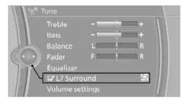
When surround is activated, multi-channel playback is simulated when playing an audio track in stereo.
