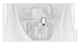
4. Using the screwdriver from the onboard vehicle tool kit, refer to page 270, press the red lever and with the button pressed, simultaneously move the selector lever to the desired position.
