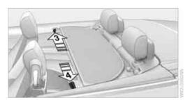
Push the fastening pin, arrow 3, into the opening provided on the right side of the vehicle until it snaps into place. Remove the protective caps beforehand, if necessary.  Push the fastening pin, arrow 4, into the opening provided on the left side of the vehicle until it snaps into place.
