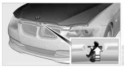
In order to avoid damage, make sure that the wiper arms are against the windshield before you open the hood. Do not open the engine hood before the engine has cooled down; otherwise, injuries may result. ◀
