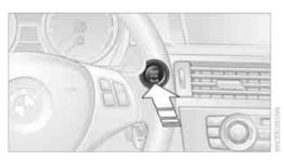
Pressing the Start/Stop button switches radio readiness or the ignition on or off.
