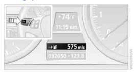
Press the button in the turn signal/high beam lever.
