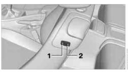
To move the front seats forward or backward from outside or from one of the rear seats; with the door open, press the front end 1 or rear end 2 of the switch.
