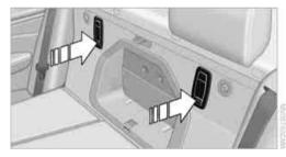
When the rear seat backrest is folded down, you will find two bag holders on the cargo area wall:
