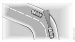
Because of the limited range of the system, it is possible that in curves or on the peaks and valleys of hilly roads, a vehicle ahead may be recognized late, or not at all. Therefore, it is up to the driver to select a speed that is prudent in view of the curves and terrain of the roadway.
