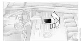
Add up to 1 US guart/1 liter of engine oil only after a corresponding message is shown on the Control Display.
