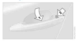
Grasp the handle on the driver's or front passenger door completely, arrow **1**. This corresponds to pressing the a button.
