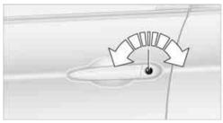
Do not lock the vehicle from the outside if there is any person inside, because the vehicle cannot be unlocked from inside without special knowledge.◀
