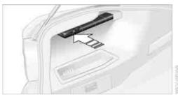
The warning triangle is located on the left-hand side of the cargo area. Press the tab to take it out.
