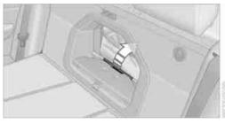
You can remove the front cover to use the full height of the through-loading opening. With the cover folded down, pull the handle, see arrow, and remove the cover toward the front. To replace, insert the cover at an angle from above and let it snap it into place.
