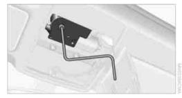
6. Reinstall the control unit and reattach the lamp cover.
