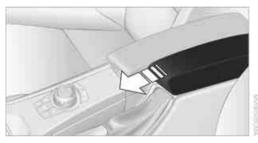
Slide the center armrest on the driver's side into the desired position.
