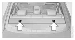
For child restraint systems with tether straps there are two additional anchors, see arrows.
