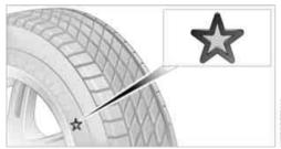
Certain makes of tire are recommended by BMW for each tire size. They are marked with a clearly visible BMW designation on the sidewall of the tire.
