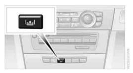
Briefly press the button in the center console to raise or lower the roller sunblind.
