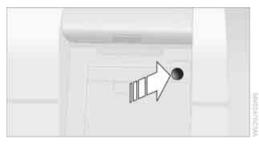
Open the Velcro fastener, spread the ski bag between the front seats and insert the skis or snowboards.
