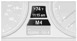
The selector lever position is displayed and, in manual mode, the engaged gear, e.g. M4.
