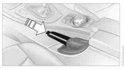
Pull slightly upwards, press the button and lower the lever.
