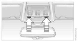
There are reading lamps at the front and rear, next to the interior lights. To switch on and off, press the button.
