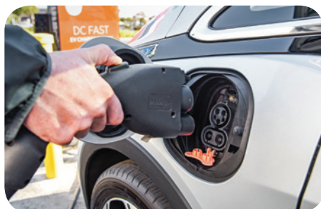
DC Fast Charging port (orange cover removed)
