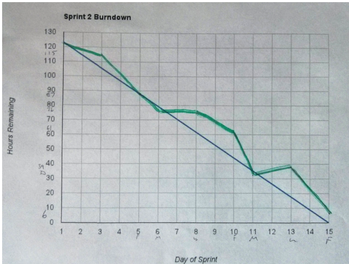
Figure 8. Burndown chart from Sprint 2, showing steady progress (straight line) vs. actual daily progress (hand-drawn line).
