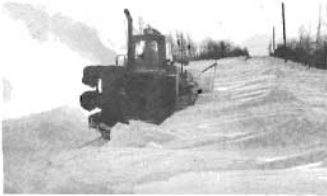
Cutting through snow with a snow-blower mounted on a Hough Loader on a minor road in the Sunrise Area, south-east of Fort St. John. Many miles are often drifted in like this because of the open farm land. The operator is Walter Daunness of Fort St. John.
