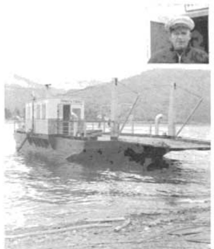
The end of a decade of operation by the Renata Ferry came February 3. Plying the Lower Arrow Lakes between Deer Park and Renata, (both of which will be flooded by the High Arrow Dam), the steel hulled vessel was formerly a freight carrying tow barge converted into a ferry under the direction of Russell Broughton, Mechanical Foreman from the Rossland Shop. Head Ferryman, John Rohn, (insert) served on the ferry from its initial runs.
