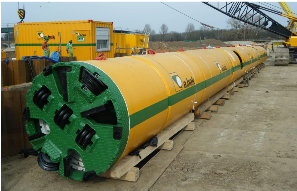
Figure 2. Adapted micro tunneling machine for the direct pipe method.
