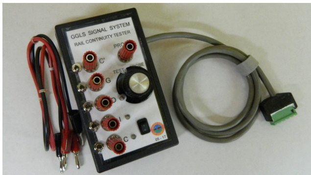
Dan Swanson – Electronic track rail continuity tester.
