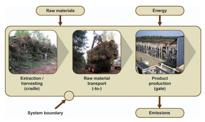
Figure 1.—Generic cradle-to-gate product production flow diagram.
