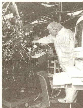
Tom Hasenberg grows a semiconductor laser with the molecular beam epitaxy machine.
