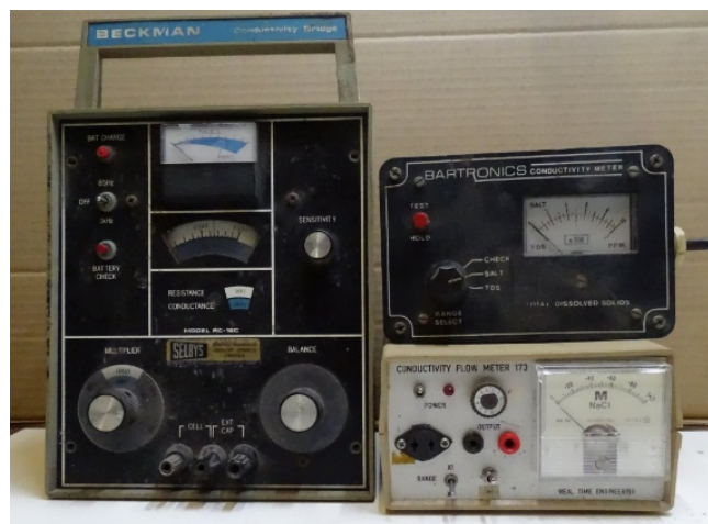
Figure 3. Illustration of two mid 1900 conductivity meters including a reference to the use of MHO
