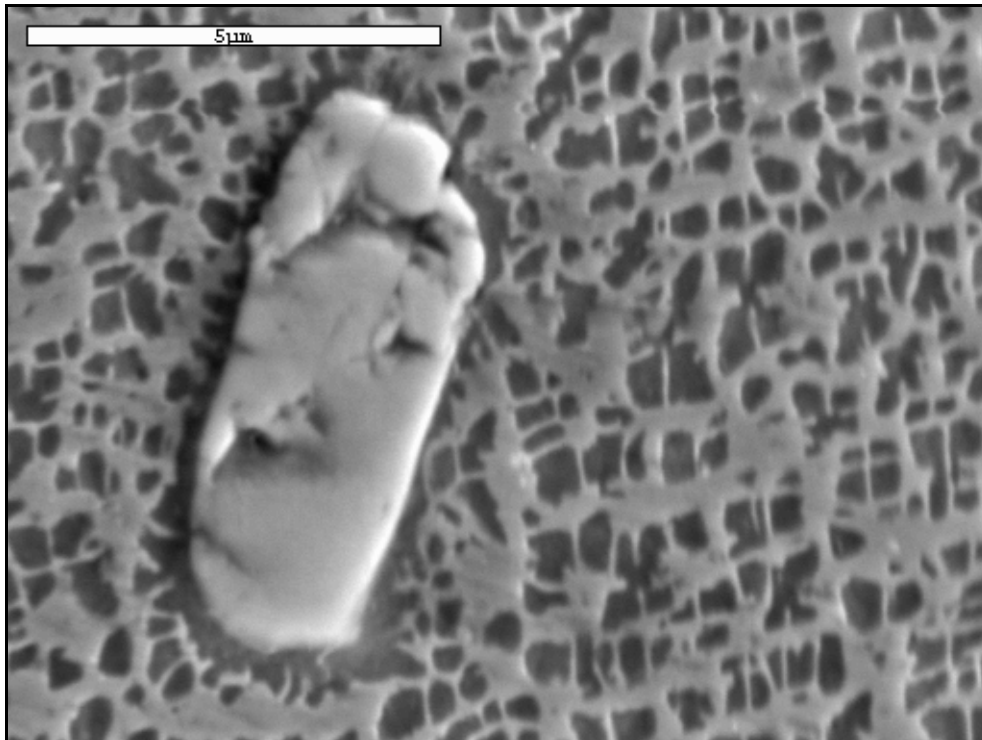
Figure 40 – SEM of MC carbide in matrix (10000X)
