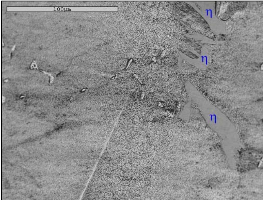
Figure 35 - BSE SEM of freckle boundary in the DS-1 showing \eta phase (500X).
