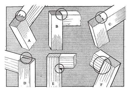
FIG. 2. THINGS TO AVOID WHEN MAKING THE MORTISE AND TENON JOINT.
