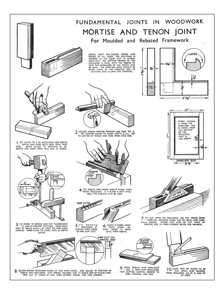
wood, the thickness of which equals that of the tenon and of a width the same as the haunch length and use this as a template. Then as you cut the socket you can try it in. When it fits in flush without a gap you know that the haunch will do the same. The simplest way of cutting is to saw down the sides with a dovetail saw and chisel away the waste.
