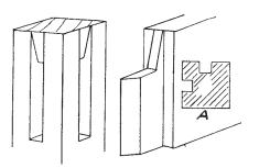
FIG. 4. BEVELLED HAUNCHES ARE STRONGER IN LIGHT TABLE LEGS
