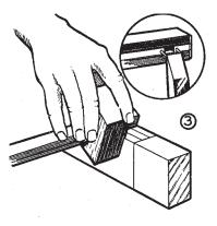
**6.** Mark tenon with gauge from face side. Fix wood at an angle to start cuts and hold saw to waste side of gauge line. Reverse and fix upright to finish (inset).
