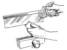
FIG. 2. FIRST OPERATION WHEN SAWING THE TENON
