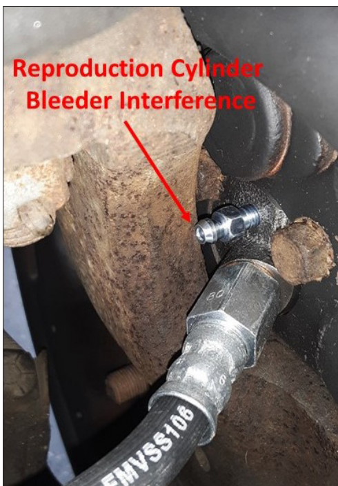
Because the bleeder screw is not angled as the original, it strikes the spindle arm.
