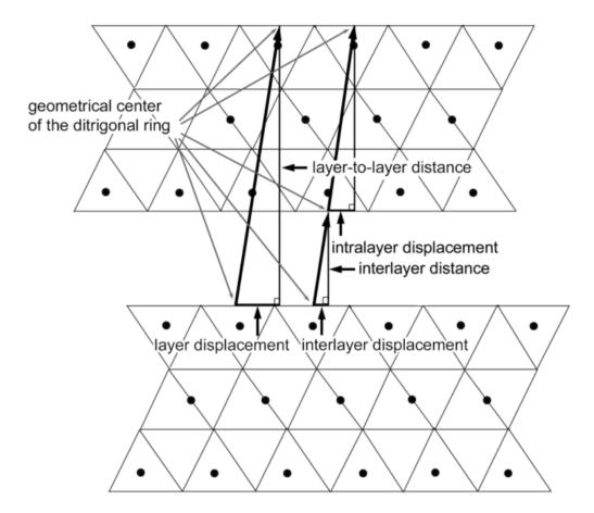
Figure 1. Illustration of terms used to describe interlayer, layers, and intralayer topologies. From Guggenheim *et al.* (2009).
