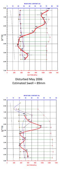
Undisturbed June 2007 Estimated Swell = 63mm New Filter Batch
