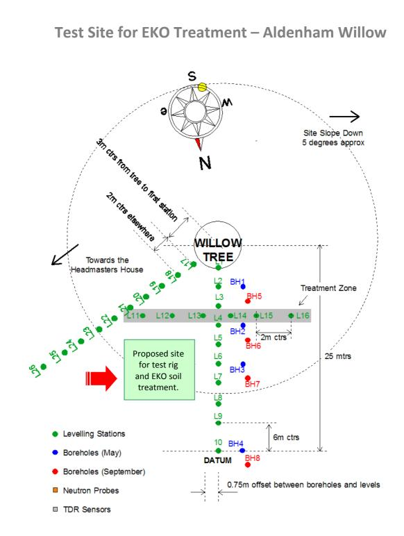
A load frame is to be installed on site at the above location (indicated by a red arrow), between the two levelling arrays. See following pages for details.
