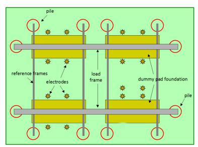
A preliminary and diagrammatic illustration of the proposed apparatus. Four concrete pads will rest onto the shrinkable clay soil, within influencing distance of the Aldenham willow. The ground beneath the pads will be treated and movement monitored using levels and pressure devices.
