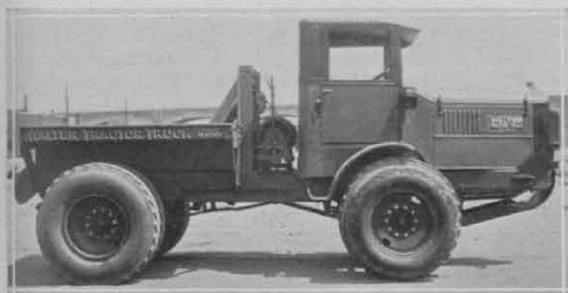
7½ Ton, 4-Wheel Drive, Walters Truck (Now Under Test)
