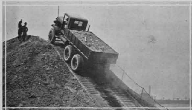
170 H. P., 6-Wheel Drive, Truck with Sterling Motor, Assembled in Army Shops
