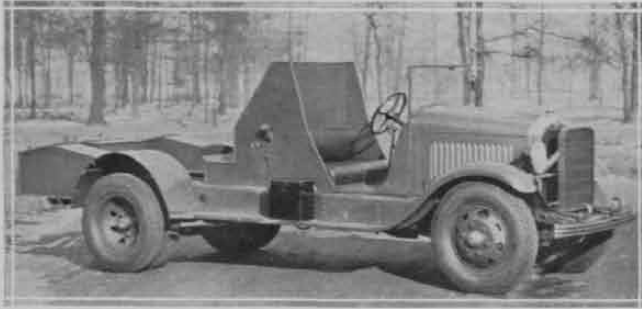
Truck Designed for AA Machine Gun. 3½ Ton, White Chassis. (Now Under Test)
