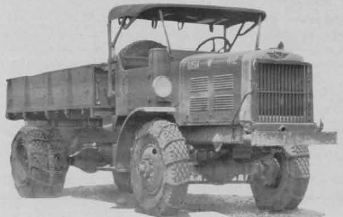
5 Ton, 4-Wheel Drive, F. W. D. Truck. (Adopted as Standard Cargo Vehicle)
