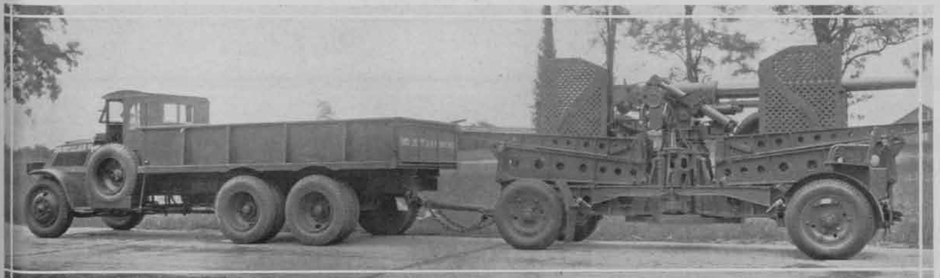
10 Ton, 4-Wheel Drive, Mack Truck, Used as a Prime Mover for the AA Gun. (Now Under Consideration for Adoption).
