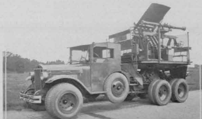
Diamond T 4½ Ton Truck Carrying Self Contained AA Machine Gun Unit
