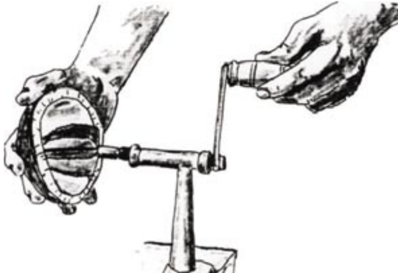
Figure 7-2. A toothed mechanical device designed to speed up the shredding of kernel from the nut.
