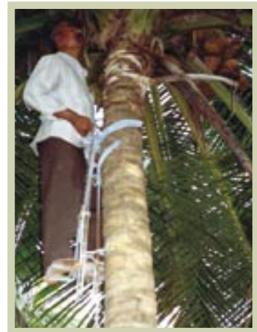
Figure 6-4. No particular fitness or climbing skill is needed to climb a palm assisted by the climbing frame.
