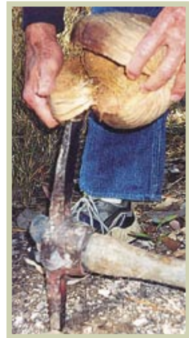
Figure 9-2. The spike of a common digging pick being employed for dehusking — convenient, but not an ideal height for comfortable use.
