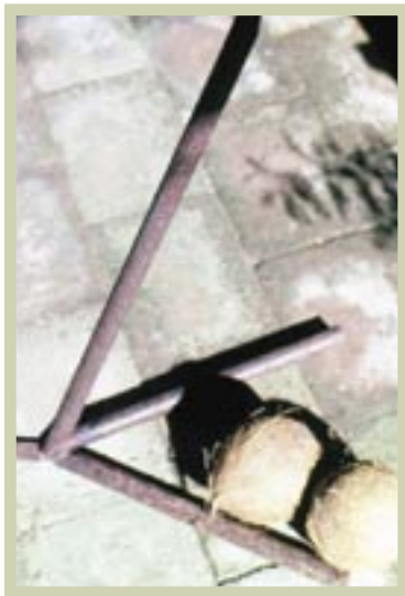
Figure 9-1. A metal dehusking pipe supported by a triangular base. The pipe may be unscrewed from the base for easy portability.
